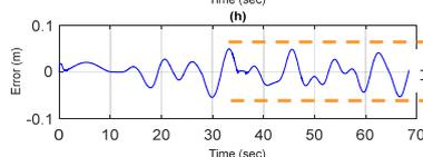
(h) Control error of 4<sup>th</sup> hydraulic cylinder position control response
