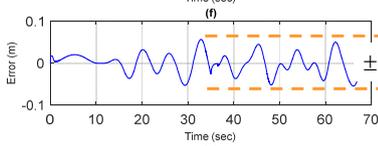
(j) Control error of 5<sup>th</sup> hydraulic cylinder position control response
