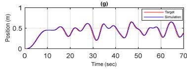
(k) 6<sup>th</sup> Hydraulic cylinder position control response
