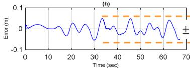
(l) Control error of 6<sup>th</sup> hydraulic cylinder position control response
