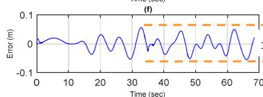
(f) Control error of 3<sup>rd</sup> hydraulic cylinder position control response
