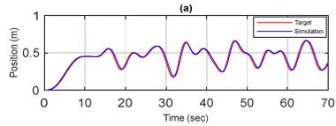
(a) 1<sup>st</sup> Hydraulic cylinder position control response
