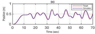
(c) 2<sup>nd</sup> Hydraulic cylinder position control response
