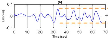
(b) Control error of 1<sup>st</sup> hydraulic cylinder position control response
