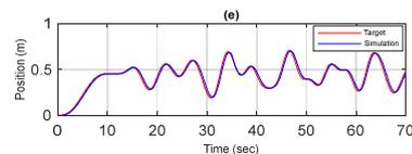
(e) 3<sup>rd</sup> Hydraulic cylinder position control response
