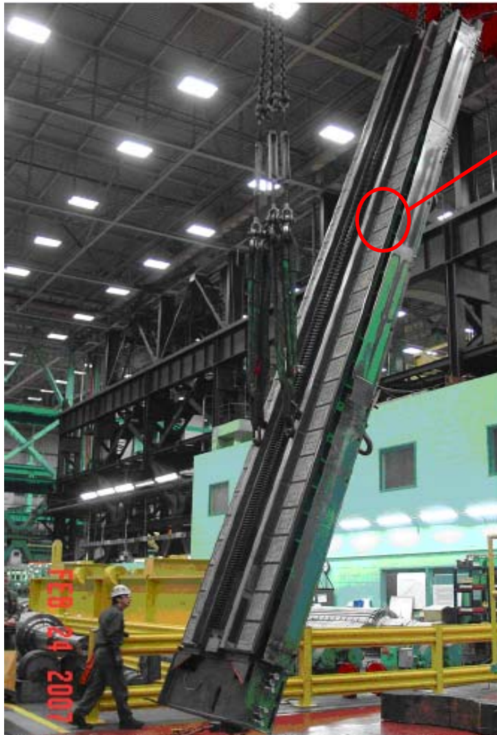
IMAGE 1. A 40 foot table segment with 30 hydrostatic bearing pads per way, being turned end over end. The table segment is fabricated from steel.
