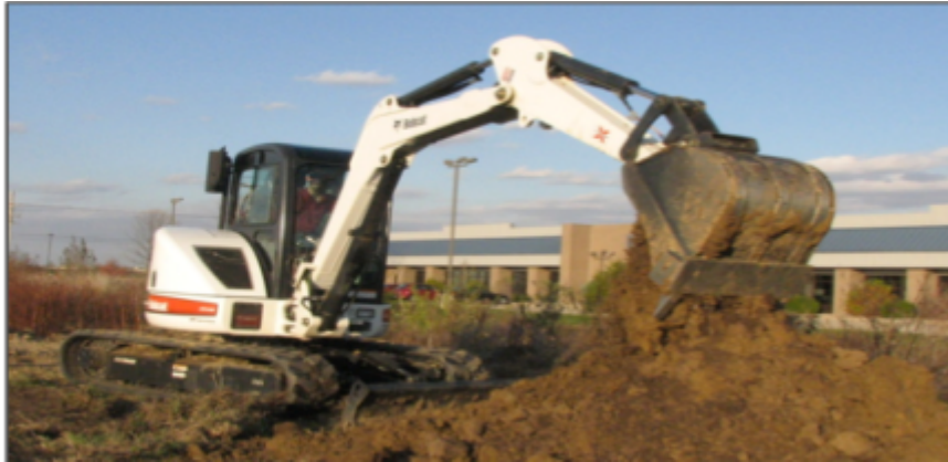
Excavator Test Bed has been fitted with variable displacement pumps
