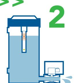
Sensor detects high water level and discharges condensate by opening the ball valve automatically.
