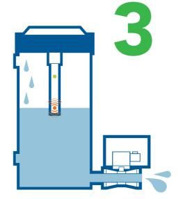
Sensor signals the valve to close when condensate discharged down to low water level.
