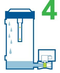
Water Seal prevents air leakage when the valve closed.
