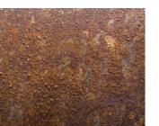
Condensate in any pneumatic circuits causes rust and coated surface shedding of the equipment. Consequently, we will have rough surfaces and particles accumulation. The humidity in the system is over 40%, the equipment will have rust. The wear speed and breakdown frequency also increase. These will severely impact the profitability of the operation.
